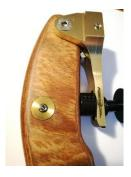
Tighten the adjusting screw until it stops: there must be no free space below the cradle.
